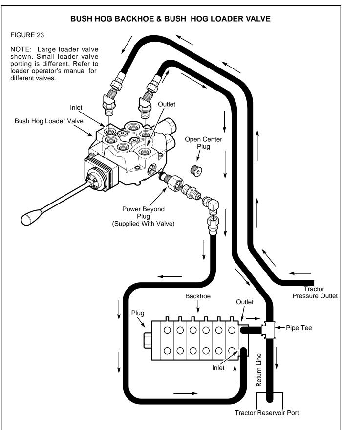
IMPORTANT: Never connect the return hose to a tractor remote coupler which can be pressurised. Accidental pressurization can cause serious damage to backhoe valve.
